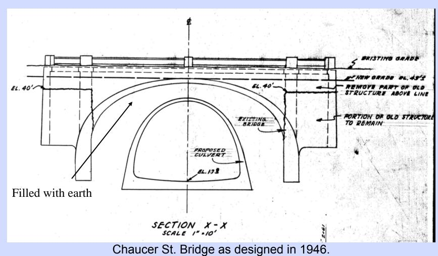
Original height on centerline (invert to soffit) = 19.5 ft; current height  $\approx$  16.5 ft
